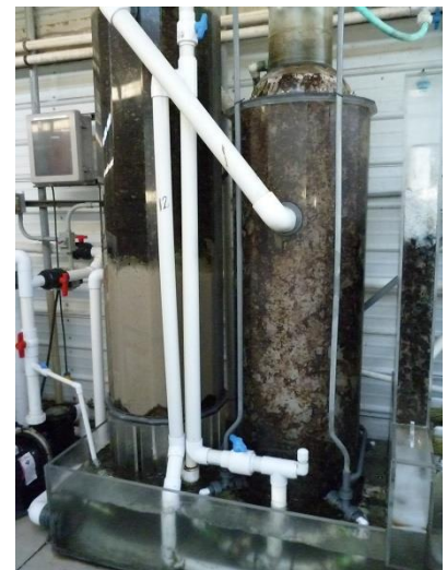
Fluidized bed filters are high performance filters with a very high filtration capacity (photo courtesy Shane Willis 2016)
